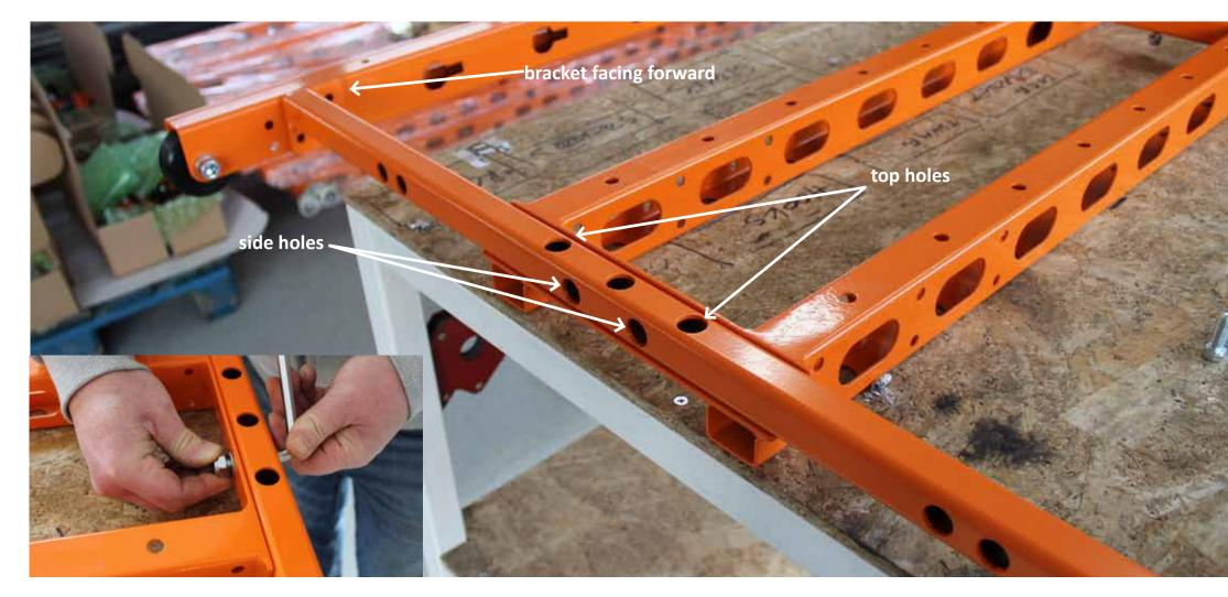
Place the rear bar with the side brackets pointing forward. The three top holes will match the three holes in the central chassis.
