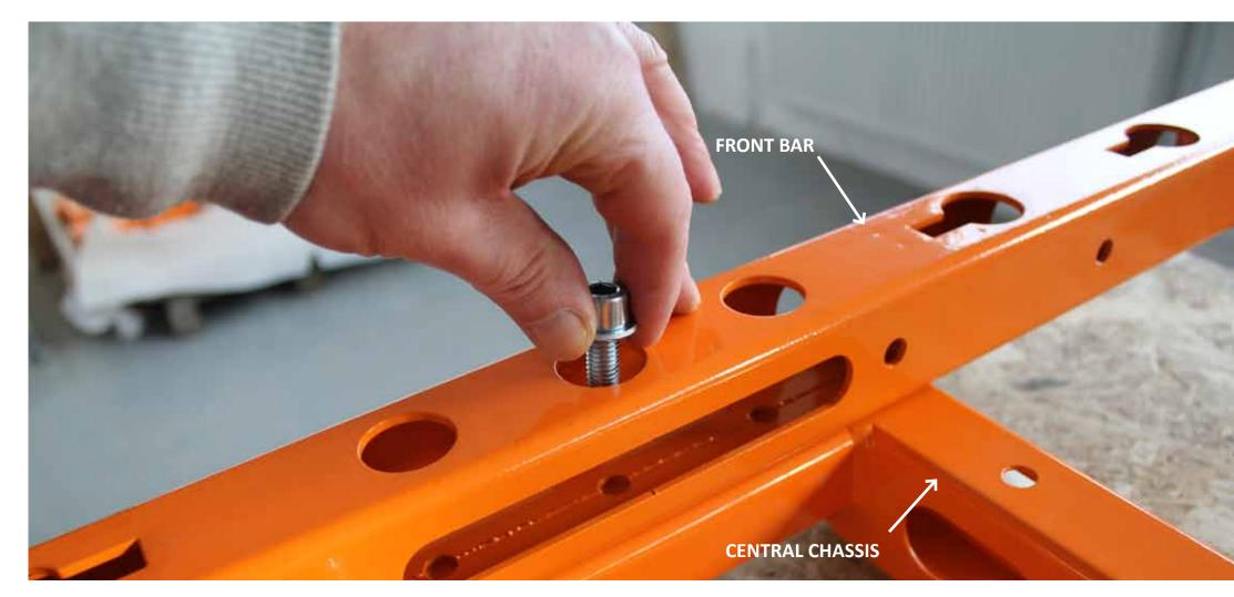
Place the front bar on top of the central chassis at the front of the chassis. There are matching holes in the front bar to match the three top holes of the central chassis. Slide the bolts through those holes.
