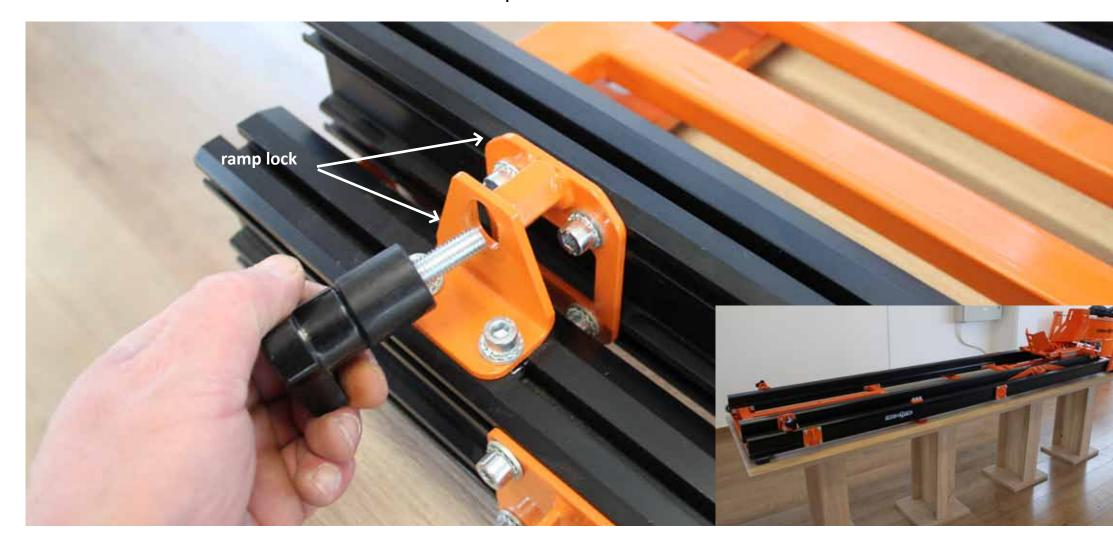
Detach both lock brackets from both sides of the ramp.
