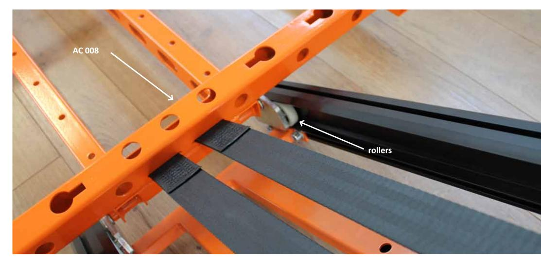
Make sure the rollers track right inside the tilt frame beams and run the ramp to raise the AC 008 about halfway up the tilt ramp.
