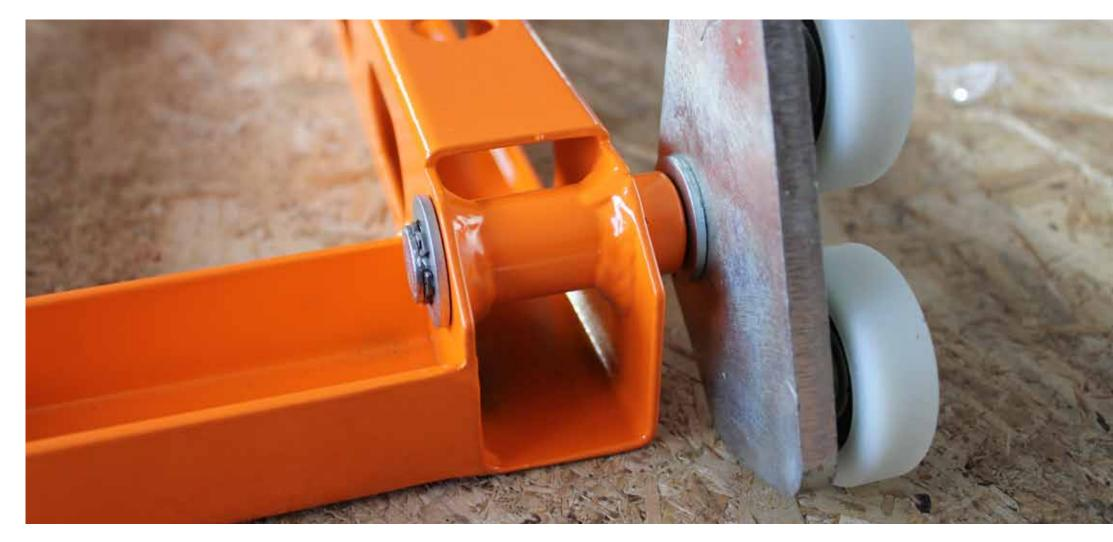
Some early kits were delivered with loose roller plates. If that is the case with your kit, use two 16mm washers and the circlips provided to attach the roller plate stub axle like in the picture.
