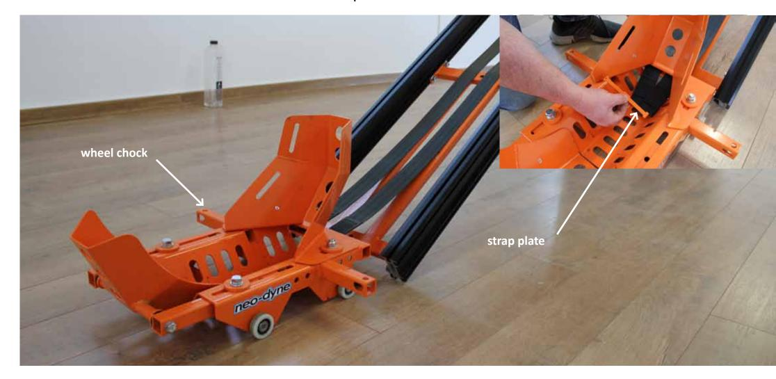
Run the ramp to discharge, slide the wheel chock off the rails. Remove the strap plate and remove the wheel chock.
