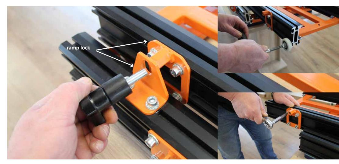
Detach both lock brackets from both sides of the bottom ramp, and also the back rollers.
